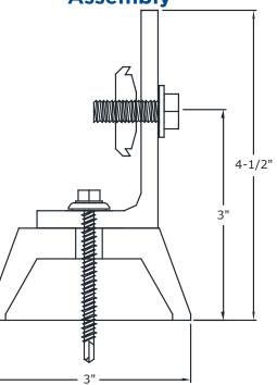
Tek Screw For Steel Roofing Members, Lag Screw For Wooden Rafters
